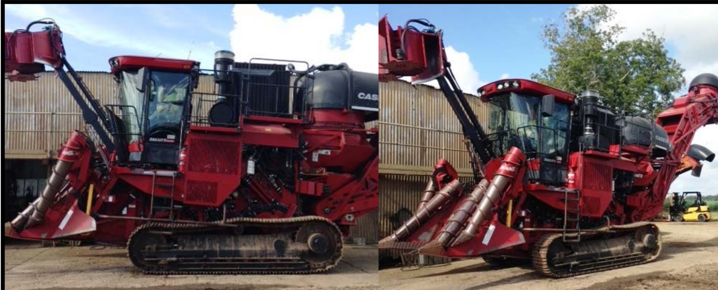
M1901- 2017 Case 8800 Harvester - Track Harvester modified for 2M rows with EHS Choppers. (1940 hours)
