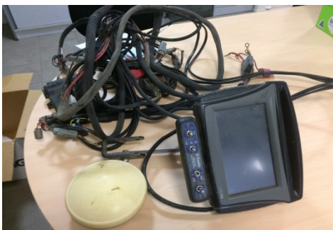
Item ST1703 – Trimble GPS fertiliser rate controller
